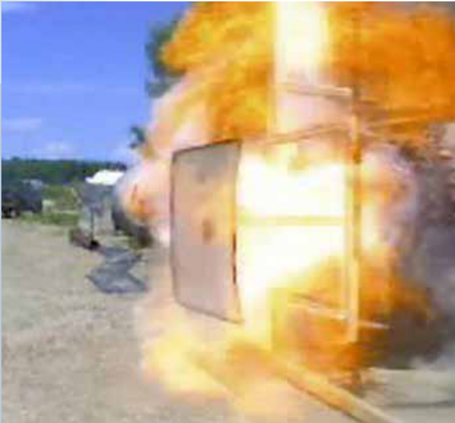
Dynamic testing of a VSB building vent
